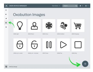
In the next screen, enter a name for the image and upload your image. The image will be automatically converted to a 200 × 200 pixel black & white image after uploading.
